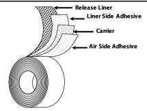
Liner:76lb bleached polycoated kraft,<br/>silicone coated on both sidesLiner Side Adhesive:Rubber (1902)Backing/Carrier:0.5 mil polyester film
